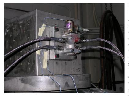
The Solenoid Sequence Valve (SSV) was bench checked and found to be within design parameters. A test rig was then designed to test its function during dynamic vibrations. This was a full 2 days at increasing vibration levels and at decreasing voltages, to ascertain when the SSV would release hydraulic pressure to the aircraft lock actuator. This type of testing had not been done during development. The component was first tested for function, put
