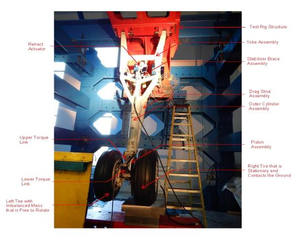
The MLG assembly test rig included:
